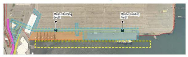
The locations of the proposed marine buildings (shown here) will provide required proximity to berthing facilities and cranes for both worker safety and convenience, and cause minimal impact to terminal layout.
